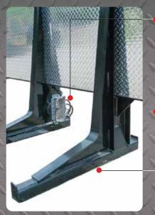
TruckLite sealed junction box mounted inside of uprights providing maximum protection from the elements. Wired and ready for truck installation.
