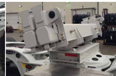
Bunks and Hydraulic Power Towers
