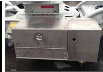
Diesel Hydraulic Power Unit
